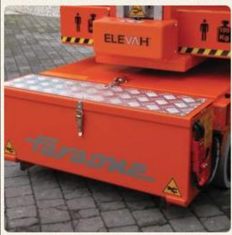
24hr charging kit comprising two box batteries and a charger.
