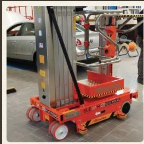
Ballast weights for polished or slippery floors
